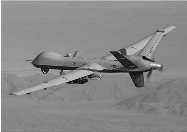
**Figure 12. MQ-9 Reaper remotely piloted vehicle**
