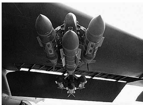
**Figure 8. Low-cost tail kits on “dumb” bombs provide precision guidance from the GPS**
